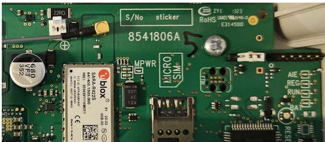
Figure 5: Installing the SIM card
