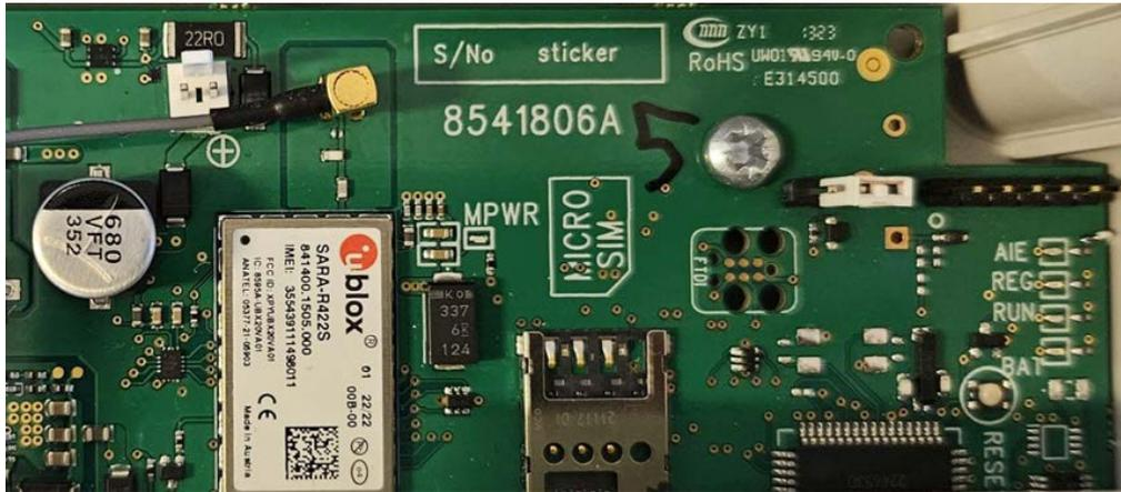
Figure 6 The antenna is connected to the MMCX connector above the radio module.
